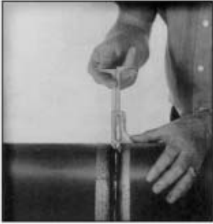
Measure internal mismatch, pipe wall.
